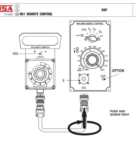
Is it possible to connect the RC1, to all  $\ensuremath{\mathsf{DSP}}$  engine driven welders.
